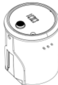
Battery pack indication LED lights
